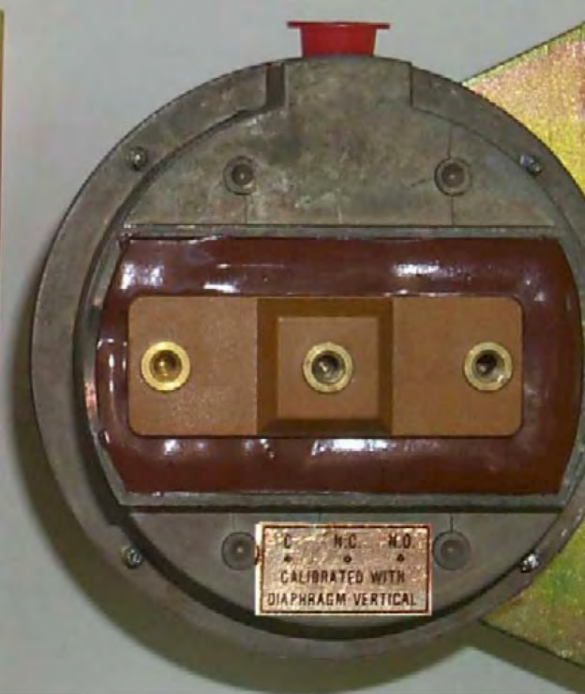
Back of Air Switch - Correct Labelling
